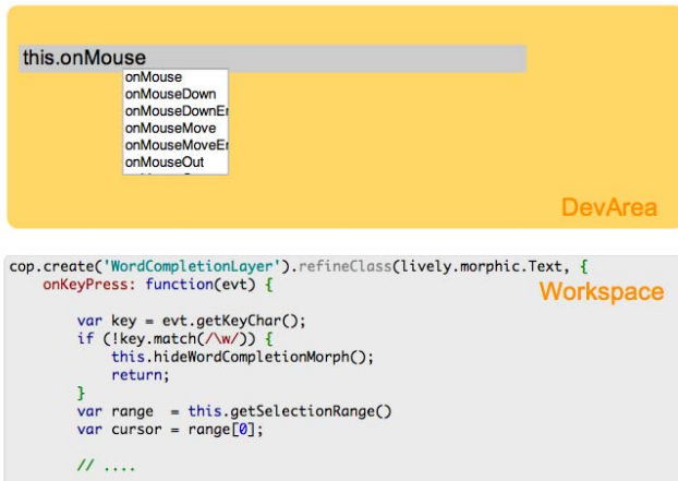
Figure 8: A snapshot of developing autocompletion of source code, showing a workspace and an area where the new code is activated.
